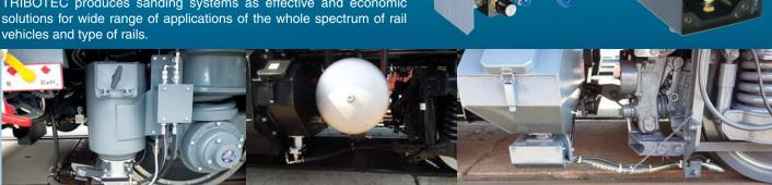
The sanding equipment for railway vehicles KOVA is a modern ecological system whose pneumatic principle ensures operational reliability. System KOVA is designed for locomotives which are equipped with their own source and distribution of pressure air.
