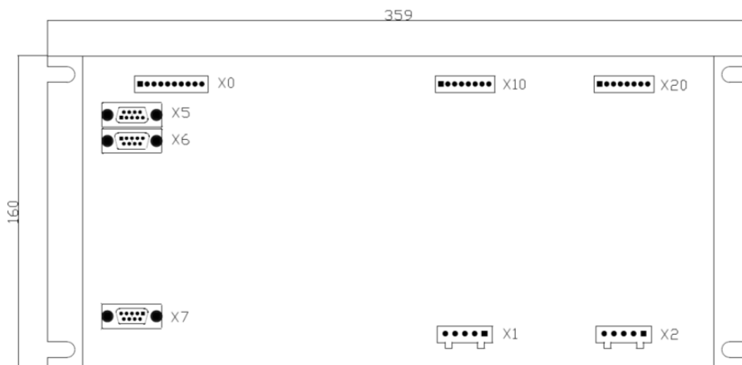
Fig. 2 The layout of connectors on the PJP-04-02 unit
